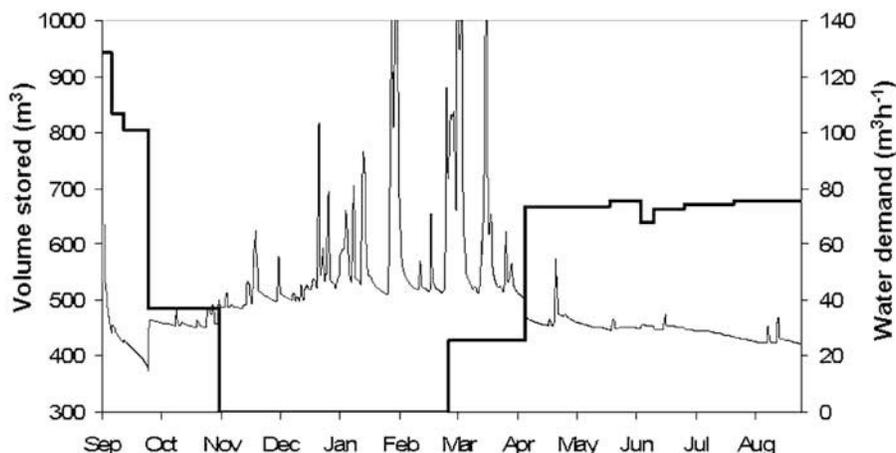
**Figure 3.** Calculated water storage (thin curve) and water diversions (bold curve) from reservoir 2 for the baseline simulation. The large fluctuations in storage are due to the small size of the reservoir with respect to the inflows. Reservoirs in the study area were built to maintain the water levels above the diversion channel and not to store water.
