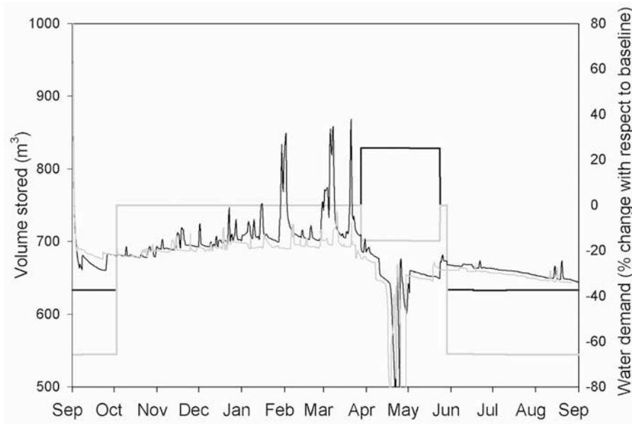
**Figure 8.** Calculated water storage in (thin curves) and change in water diversions from reservoir 5 with respect to the baseline case (bold curves) for the 25% precipitation reduction (black lines) and 50%.
