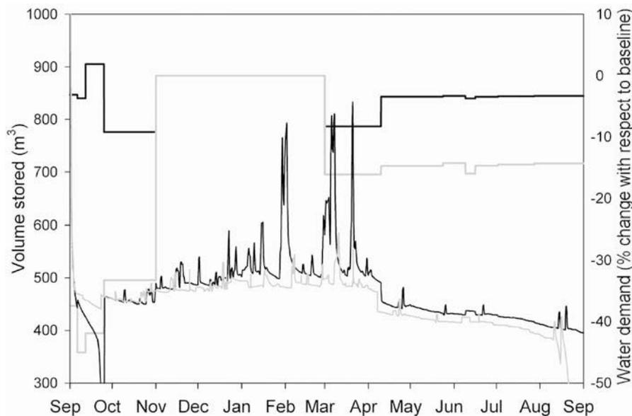
**Figure 5.** Calculated water storage (thin curves) and change in water diversions from reservoir 2 with respect to the baseline simulation (bold curves) for the 25% precipitation reduction (black lines) and the 50% precipitation reduction (gray lines) scenarios. The large fluctuations in storage are due to the small size of the reservoir with respect to the inflows. Reservoirs in the study area were built to maintain the water levels above the diversion channel and not for water storage.
