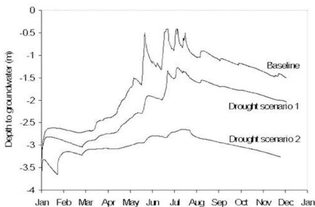
**Figure 7.** Depth to the water table in one of the wells used by farm 4.
