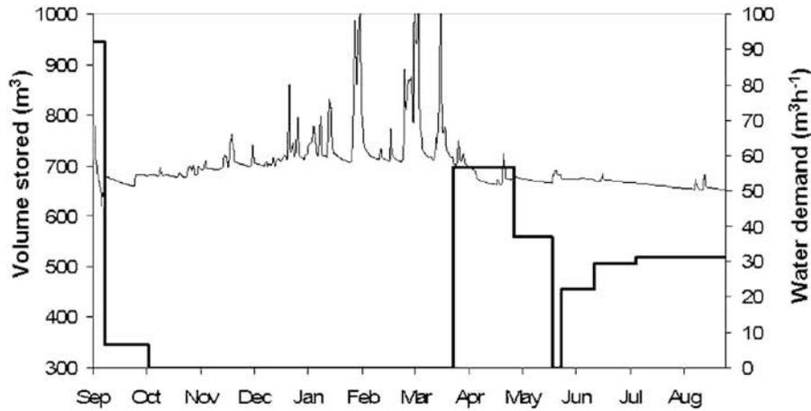
**Figure 4.** Calculated water storage (thin curve) and water diversions (bold curve) from reservoir 5 for the baseline simulation. The large fluctuations in storage are due to the small size of the reservoir with respect to the inflows. Reservoirs in the study area were built to maintain the water levels above the diversion channel and not for water storage.
