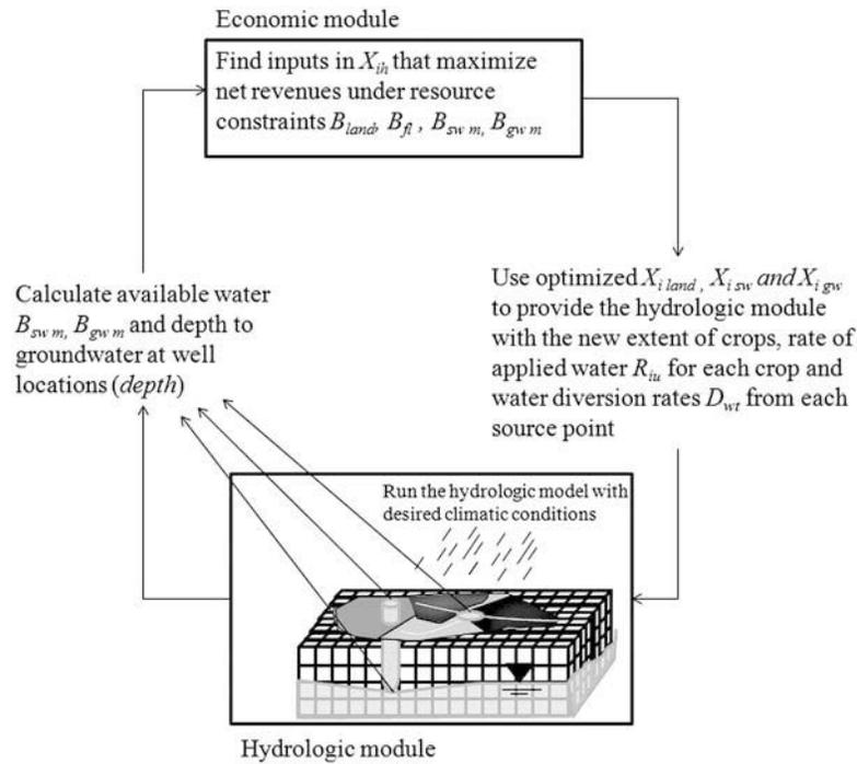
**Figure 1.** Schematic of the loop between the hydrologic and the economic model of agriculture. The modules iterate until the economic model converges to a state that is consistent with the available resources.
